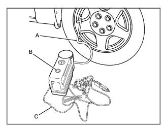
Attach the sealant filling hose (A) onto the tire valve stem. Turn it clockwise until it is tight.
